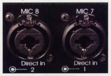
Channel 7 & 8 Neutrik combo connectors double as mic (XLR) and instrument DI (1/4") inputs. When a 1/4" plug is inserted, a small relay is activated to switch the active DI circuit into the signal path.
